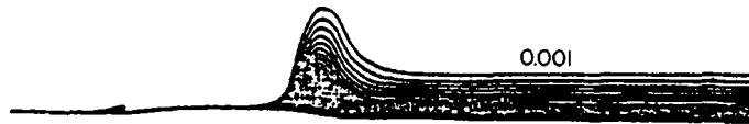
Figure 4. GAMM channel with circular bump; isentropic lines (increment \Delta S = 0.001 ) (one step upwind method)
